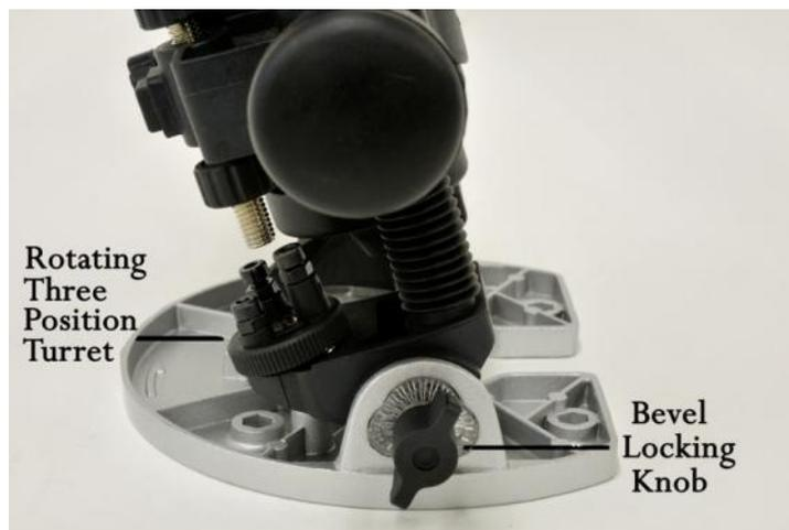
**Note: Depth of cut will usually have to be increased after tilting the router base for bevel cutting.**
