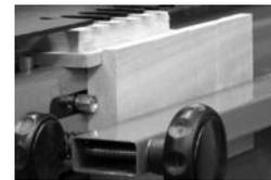
10) Remove the gauge block from under the front clamping bar
