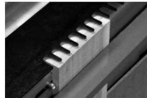
***TIP: If you'd like to make future setup faster and easier, the setup board can be routed in the same position as the drawer front and then used in the future to set the bit height.***
