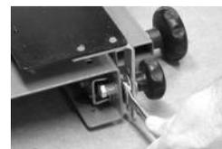
13) Attach the 5/8" diameter guide bushing to your router base.
