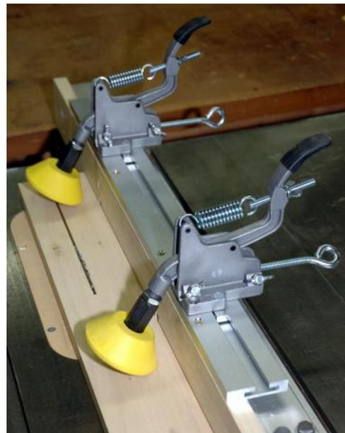
**Fig 3. Feed Safe Installation with Optional Mounting Track**
