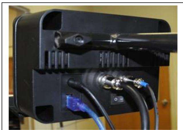
5. The control box has a shelf on it to hold your android device if you choose to set it up this way. Now you can connect your android device to the control box using the USB cable and micro adapter if needed. Your device should recognize you are connected to the lift when opening the MLCS PowerLift Pro App.
