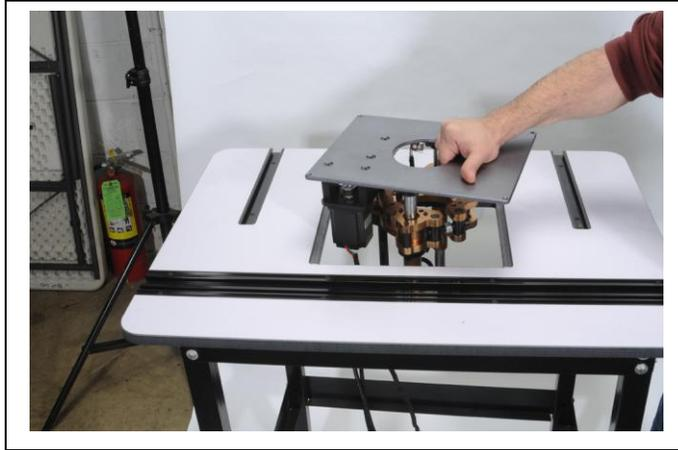
2. If you cannot rotate it into position the lift carriage will need to be lowered down the guide posts. Follow the instructions on connecting the cables to the foot pedal and electronic control box(ECB). Once the cables and power are connected you can simply use the foot pedal and press down to lower the carriage (no android device is needed here). It is also easier to install the router motor with the carriage in its lowest position.
