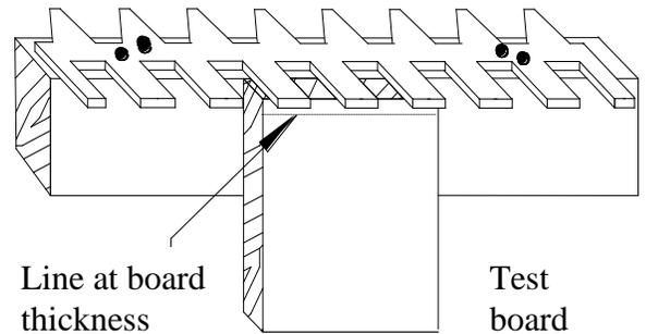
Move template with reference to mounting block
