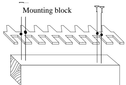
the face of the test board is clamped to the face of the mounting block. The straight fingers should be sticking out over the end of the test board, facing you.
