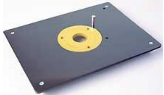
Locate the top/front of your base plate by observing the position of the starting pinholes. The holes will be to the **RIGHT** of the bit opening. Again mark with tape front and center on the plate to serve as a reminder.
