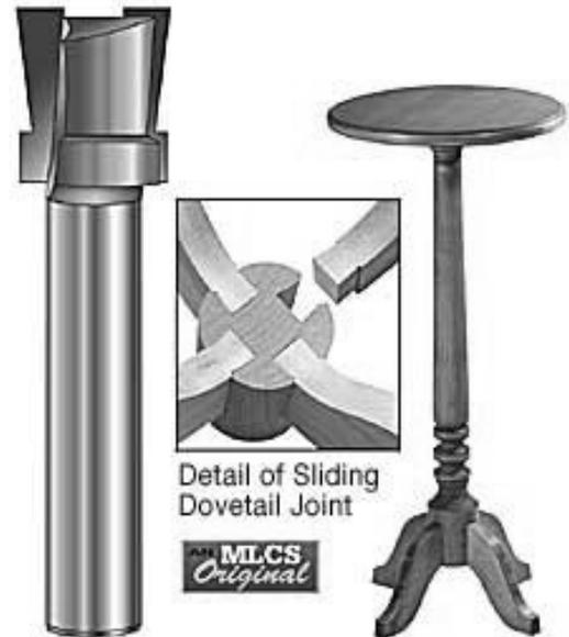
10. Switch to the Candle Stand bit, but leave the fence and stop blocks in the same position. Adjust the bit height so that you cut the dovetail and enough of the straight cutter to mortise the leg into the center post by at least 1/16".
