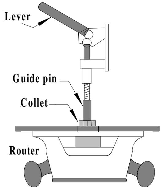
Mark the four mounting holes on your router table. Drill these holes carefully with a 3/8" bit. Install and tighten the four bolts, washers and nuts provided. Loosen the router collet and raise the pin. Your Pin router is now ready for use!
