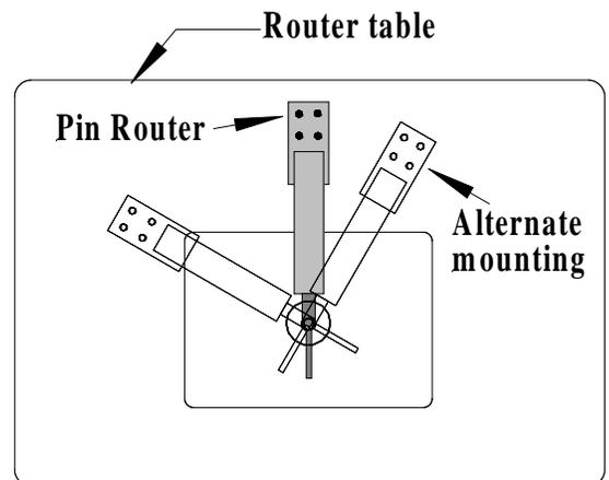
An outside pattern consists of the desired shape cut out of 1/2" or 1/4" plywood or hardboard, mounted to a backer board. The backer board should be big enough to hold and feed through the router bit. Make the pattern shape by cutting it out on with a bandsaw or jig saw, then sanding or filing the edges perfectly smooth. Any bumps or roughness on the pattern will be transferred to the workpiece, so take your time on this step.
