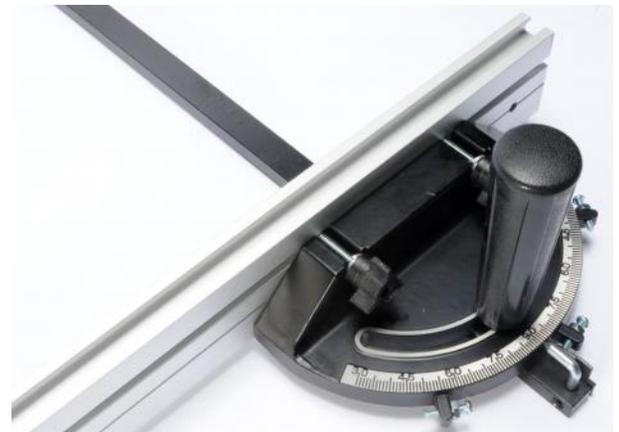
Slide the two hex head bolts into the T-Slots located in the back of the Miter T-Fence. Position the Miter T-Fence so that it will not contact the cutting blade when the Miter Gauge is pushed through its slot. The bolt should be seated into the "U" shaped slot in the Miter Gauge body. Secure the Miter T-Fence in place using a lock washer and star knob on each bolt.
