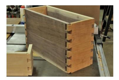
5. Using the Plywood Straight Bit set (#8376/6076), make a 31/64" dado, 1/4" deep on the inside back of the nightstand box for the plywood back. Make this dado 3/4" from the back edge of the nightstand box.
