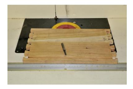
13. Use a 25/32" straight bit (#7782/5482) to create a dado on the outside drawer sides 25/32" wide and 1/8 deep, in the center of the drawer box side to receive the runner.
