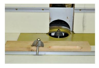
12. Create a dado in the bottom of the drawer pieces to accept the 1/4" plywood bottom panel. Use the 13/64" bit from the Plywood Straight Bit (#8376/6076). The dado should be 3/8" from the bottom edge.
