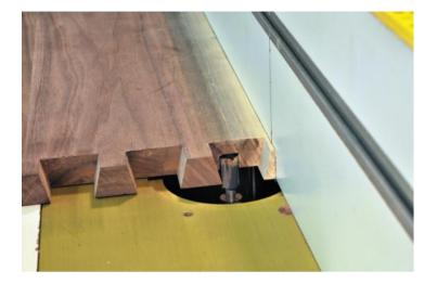
6. Cut a 3/4" wide and 1/8 deep stopped dado in the center of the inside of the cherry sides, going from front to back, using the 3/4" straight bit (#7779/5479). Start the dado at the back where the plywood dado was cut in the previous step and stop the dado 2-1/2" from the front of the side piece.
