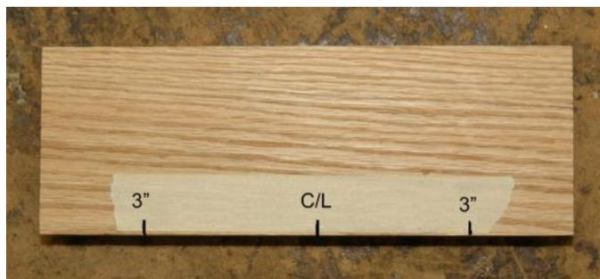
Lay both side frame pieces side by side and mark the dado layout lines on them. Transfer the layout line onto each edge of each side frame piece so that the layout lines will be visible when the inside faces are face down on the router table surface. With the 1/2" Straight Bit in the router table, adjust your fence so the 1/2" Straight Bit is centered with the shelf dado layout lines.
