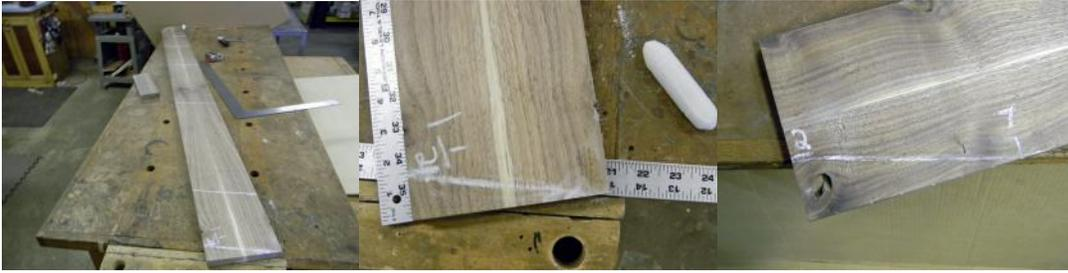
Using the remaining pieces from the uprights, make 4 backs for each shelf by ripping and crosscutting them to 2-5/8" wide x 24" length. Cut 24" off of another board and rip to 2-5/8" for the last shelf back.
