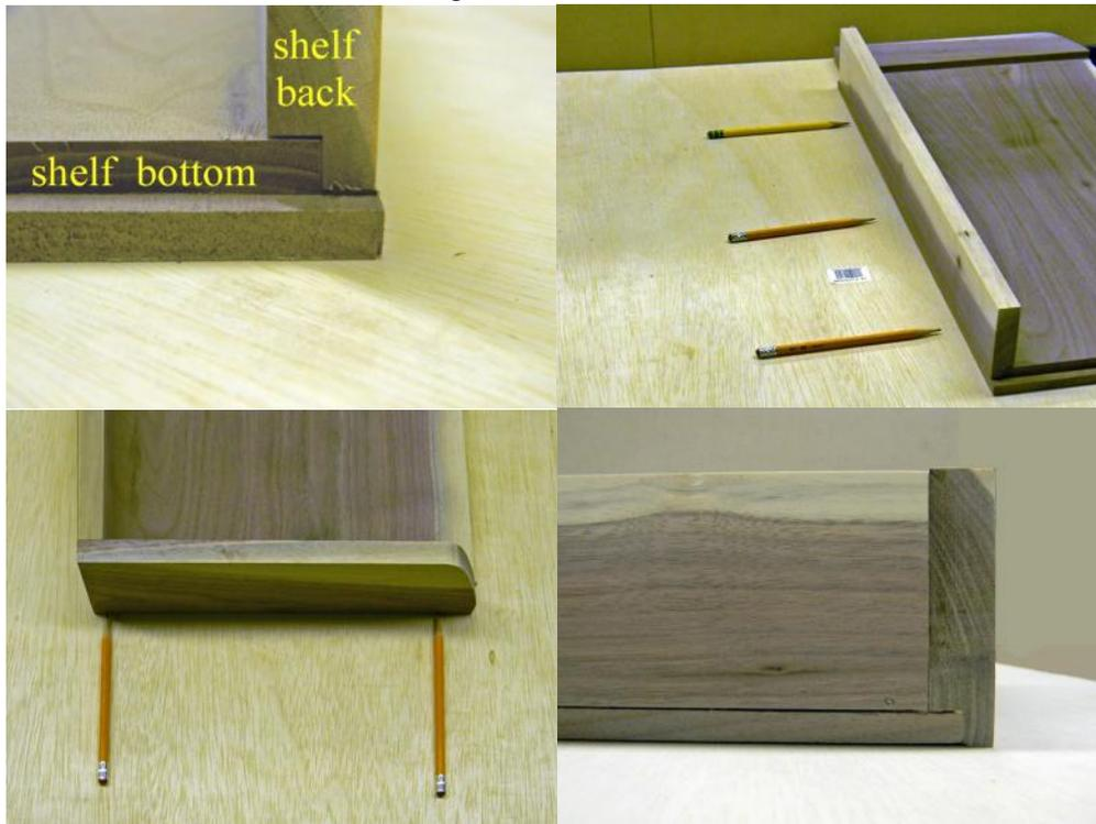
Using the 14-degree angle from the uprights, set the fence on the Router Table Crosscut Sled (#9779) for one upright. Mark on the wood where the shelves will be dado-ed into the upright. Invert the angle of the fence to cut the dados on the other upright.
